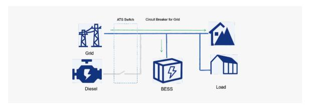
During normal grid operation, the ATS grid-side switch is closed and the diesel side is disconnected, at which time the loads operate normally and the energy storage is in charging or standby mode.
