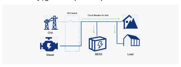
When the diesel generator is running normally, the Diesel generator side of the ATS switch is closed, the grid circuit breaker is closed, and the energy storage system is charged, at which time the diesel generator provides the load with a long period of guaranteed power. When the grid returns to normal, the ATS will disconnect the diesel side switch and close the ATS grid test switch
