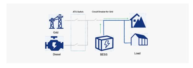
When the power grid is abnormal, the ATS disconnects the grid switch, the grid circuit breaker is disconnected, and the energy storage system provides emergency power for the load, reserving time for the diesel to start up startup
