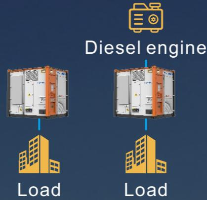
The system has been upgraded to VSG technology, enabling multi-unit parallel and off-grid use without parallel lines, which can cover a wider range of power and capacity.
